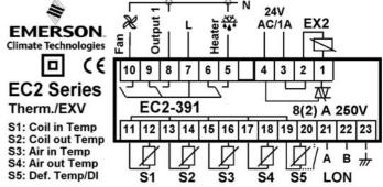
EC2 analog inputs are for dedicated sensors only and should not be connected to any other devices. **Important:** Keep controller and sensor wiring well separated from mains wiring. Minimum recommended distance 30mm.
